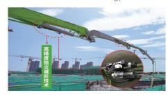
6 booms truck pump owns higher placing height and range.
